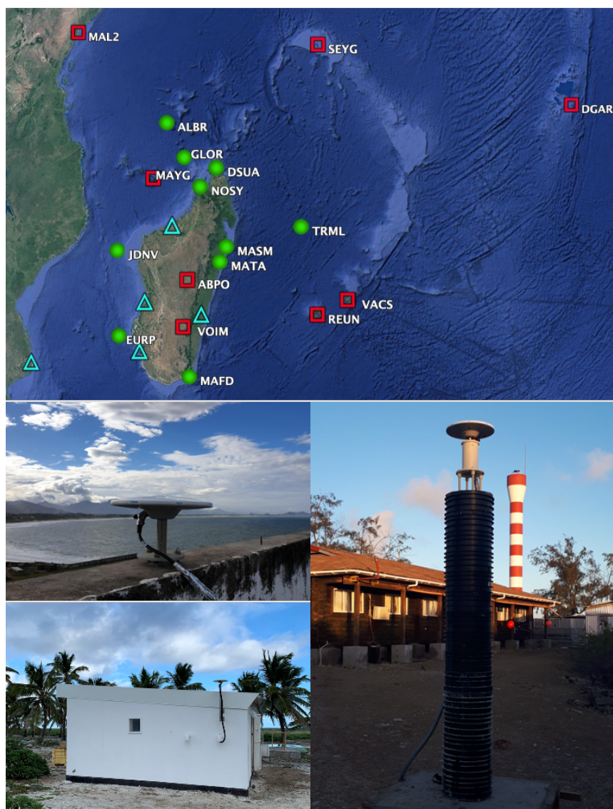
Figure 20: Map of public GNSS stations available in the SWIO as of March 2021 (top). Red squares show current IGS stations, green dots show GNSS stations installed during RNR-CYC and blue triangles show stations to be installed in 2021 in the frame of the newly project ESPOIRS (see Section 4). Pictures show GNSS stations installed in Fort-Dauphin (MAFD, upper left), Tromelin (TRML, lower left) and Aldabra (ALBR, lower right).
