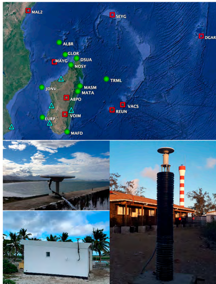
Figure 21. Map of public GNSS stations available in the SWIO as of March 2021 (top). Red squares show current IGS stations, green dots show GNSS stations installed during RNR-CYC, and blue triangles show stations to be installed in 2021 in the frame of the new project ESPOIRS (see Section 4). Pictures show GNSS stations installed in Fort-Dauphin (MAFD, upper-left), Tromelin (TRML, lower-left) and Aldabra (ALBR, lower-right). Sources: Google Earth (top); Olivier Bousquet (pictures)
